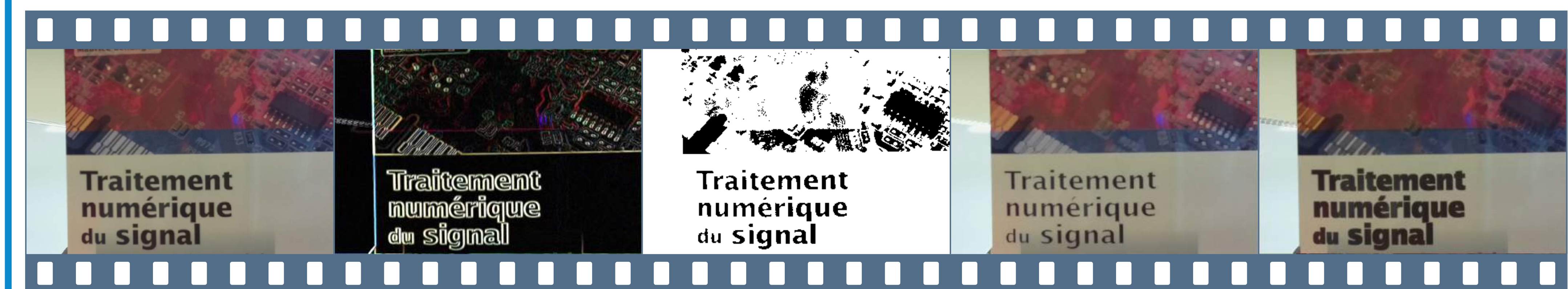
Image RGB Sobel Seuillage Dilatation Erosion
